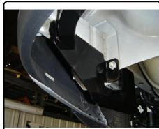
4. Fishwire 7/16-14 x 1 1/4" carriage bolt and SP7 spacer through upper and lower hole in the bumper bracket and out the rear-most hole in hitch, both sides.
