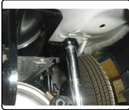
7) Raise the exhaust back into position and reinstall the rubber isolators.
