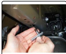
7. (2010 models only) Fishwire (1) 3/8 x 2" carriage bolt and (1) SP-18 spacer though access hole and into the upper outside hole on driver side frame rail and hitch. Place (1) SP-52 spacer and exhaust hanger onto carriage bolt and secure with 3/8" flange nut. (See EXHAUST HANGER HARDWARE ORIENTATION on page 2)
