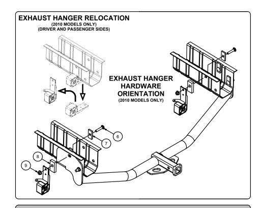
1. Remove the rearmost rubber isolator on both mufflers. Note: If installing on a 2010 model skip to STEP 2.
