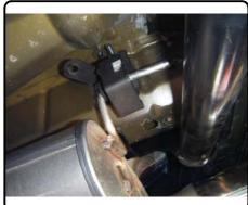
9. Torque all 3/8" hardware to 45 ft/lbs and all 7/16" hardware to 70 ft/lbs. Re-install exhaust.
