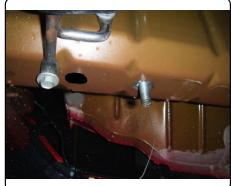
5. Raise hitch into position, being careful not to push the carriage bolts back into the frame rails. Loosely attach hitch with (2) 7/16" flange nuts.
