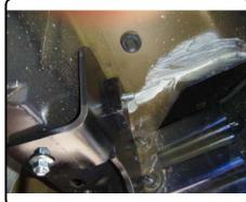
8. (2010 models only) On the passenger side frame rail fishwire (1) 3/8 x 2" carriage bolt and (1) SP-18 spacer into the upper hole on the inside of frame rail. Place (1) SP-52 and exhaust hanger onto bolt and secure with 3/8" flange nut. (See EXHAUST HANGER HARDWARE ORIENTATION on page 2)
