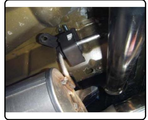
9. Torque all 3/8" hardware to 45 ft/lbs and all 7/16" hardware to 70 ft/lbs. Re-install exhaust. Install is complete.
