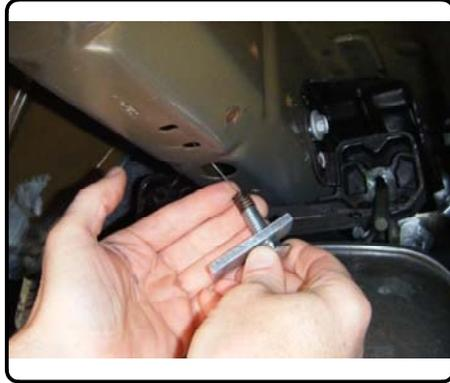
7. (2010 models only) Fishwire (1) 3/8 x 2" carriage bolt and (1) SP-18 spacer through access hole and into the upper outside hole on driver side frame rail and hitch. Place (1) SP-52 spacer and exhaust hanger onto carriage bolt and secure with 3/8" flange nut. (See EXHAUST HANGER HARDWARE ORIENTATION on page 2)
