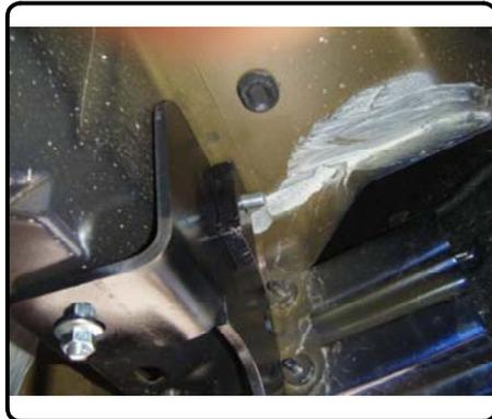
8. (2010 models only) On the passenger side frame rail fishwire (1) 3/8 x 2" carriage bolt and (1) SP-18 spacer into the upper hole on the inside of frame rail. Place (1) SP-52 and exhaust hanger onto bolt and secure with 3/8" flange nut. (See EXHAUST HANGER HARDWARE ORIENTATION on page 2)
