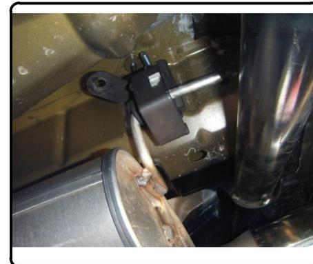
9. Torque all 3/8" hardware to 45 ft/lbs and all 7/16" hardware to 70 ft/lbs. Re-install exhaust. Install is complete.
