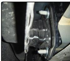
4. Lift the hitch into position over studs and secure with existing 12mm flange nuts.
