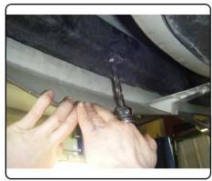
5. Fishwire 1/2-13 x 2" carriage bolt and SP6 spacers through access hole between the fascia and the back of the bumper beam and out the holes drilled in STEP 4. Raise hitch back into position and secure with 1/2-13 flange nuts.
