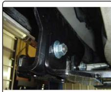
4. Press hitch against the bottom of the bumper beam. (NOTE: Be sure hitch is centered on vehicle.) Using the hitch as a template mark hole locations. Lower hitch and drill marked locations. (NOTE: Start with a small drill bit for pilot hole. A die grinder with a cone shaped bit may be easier than drill bits.)
