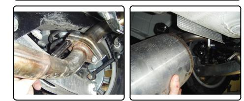
4. Remove heat shields from driver and passenger side. Return heat shields and fasteners to owner.
