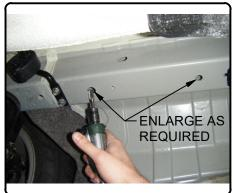
6. Fishwire 1/2-13 x 1 1/4" carriage bolts and SP6 spacers through the enlarged access hole and out the rear-most hole.
