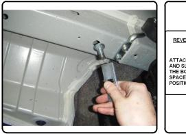
REVERSE PULL FISHWIRE TECHNIQUE ATTACH FISHWIRE TO CARRIAGE BOLT AND SLIDE SPACER ONTO FISHWIRE. PUSH THE BOLT THRU THE HOLE FOLLOWED BY THE SPACER (AS SHOWN). PULL BOLT BACK INTO POSITION, PROTRUDING FROM THE FRAME
