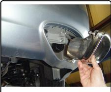
2. Remove rubber isolators from mufflers.
