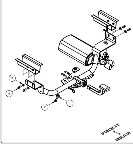
1. Lower exhaust by removing (2) rubber isolators from exhaust.
