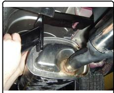
4. Loosely secure hitch with M10-1.25 x 25mm hex bolts and 3/8" conical toothed washers through existing weldnuts in outside of frame rails.
