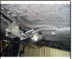
6. Torque 1/2" hardware to 110 ft-lbs and 10mm hardware to 48 ft-lbs. Raise exhaust back into position.
