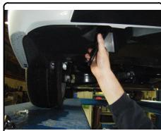
4. Mark heat shield for trimming and confirm fit. Trim heat shield using aviation shears and reinstall.
