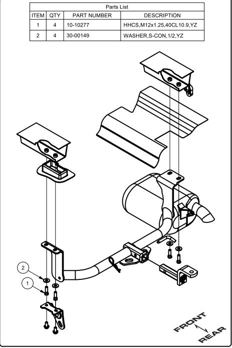
1. Remove (4) exhaust hangers and lower the exhaust, support as needed to prevent damage.
