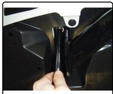
6. Raise the passenger side plate against the frame rail and secure with M12 - 1.25 X 40mm bolts and 1/2" conical toothed washers into existing weldnuts.
