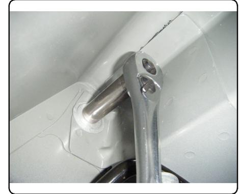
6. Raise hitch into position and attach to existing posts using the nuts that were removed in step 5.
