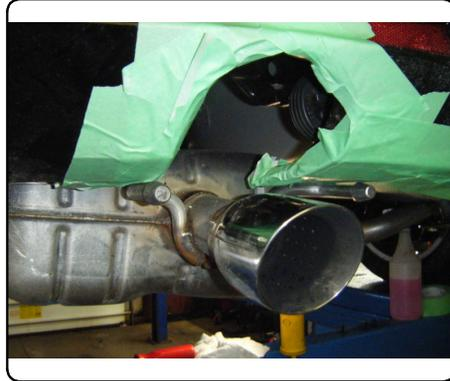
4. Enlarge access hole on driver side frame rail to allow included hardware to pass through.
