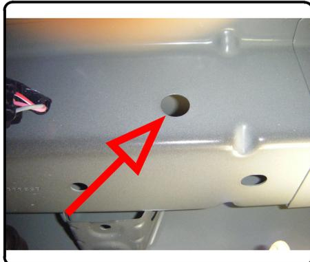
5. Remove nut from the post which is located on the inside of the frame rail, above the exhaust hanger, on the rearmost part of frame. Remove this nut from both sides.
