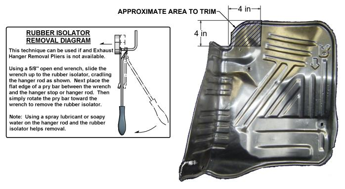
HEAT SHIELD TRIM DIAGRAM (BOTH SIDES)
