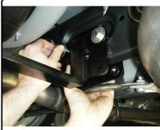
2. Raise hitch weldment past fascia lip and secure to mounting strap using 1/2-13 x 1 1/4" carriage bolts and 1/2-13 flange nuts.
