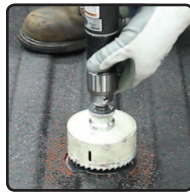
Use the pilot hole for error-free drilling
