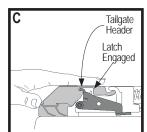
Rotate tailgate header down until both latches engage. Listen for double click.
