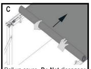
Roll up cover. Do Not disengage hook fastener prior to rolling up
