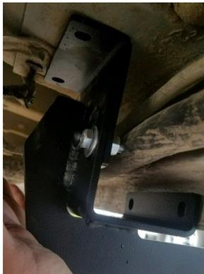
After assembling the AC bracket place along the pinch seam using Fig. 2 and Fig. 4 marking the 4 hole locations
