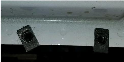
Slide 2 clip nuts on the pinch weld for lower holes attach the AC bracket using (2) 8MM Bolts and (2) 5/16 Lock Washers on the bottom Clip Nuts and (2) 5/16 Thread Cutting Bolt and (2) 5/16 lock washers on the upper holes
