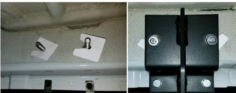
Using the 3" U-Bolt put it through the top 2 mounting holes and secure with (2) plastic bolt retainer.
