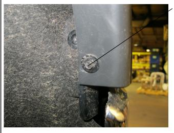
1. ON EACH SIDE OF THE VEHICLE, REMOVE THE SCREW THAT SECURES THE WHEEL WELL TRIM TO THE BODY.
