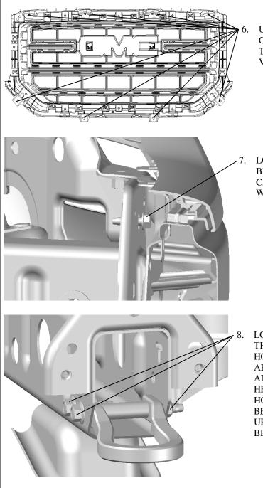
UNSCREW THE FOUR SCREWS ON THE TOP OF THE GRILLE AND THE FOUR SCREWS AT THE BOTTOM OF THE GRILLE THAT ARE SECURING THE GRILLE TO THE VEHICLE. REMOVE THE GRILLE.
