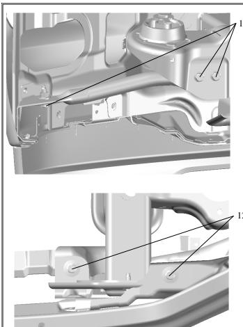
11. UNDER THE VEHICLE, LOCATE THE TWO TUBULAR SIDE BRACES AND REMOVE THE BOLTS HOLDING THE BRACE TO THE FRAME AND THEN THE OUTER BOLT HOLDING THE BRACE TO THE BUMPER. THE BRACE SHOULD BE ABLE TO BE PIVOTED TO CLEAR THE BUMPER.
