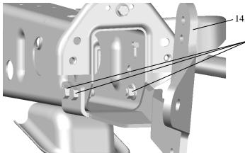
14. INSTALL THE MOUNTING BRACKET (ITEM #2 & #3) ON TO THE END OF THE FRAME. FASTEN WITH THE M12 X 1.75 X
