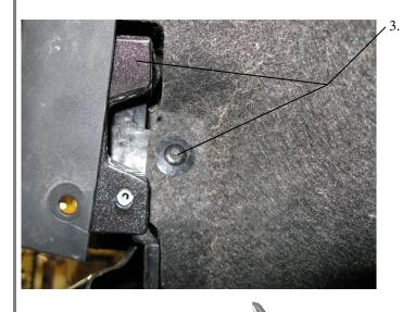
ON EACH SIDE OF THE VEHICLE, REMOVE THE TWO SCREWS THAT SECURE THE ENDS OF THE PLASTIC TRIM ON THE TOP OF THE BUMPER TO THE BODY SHEET METAL.
