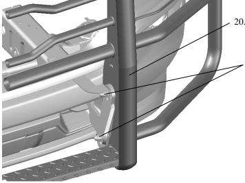
20. INSTALL THE GRILLE GUARD WELDMENT ONTO THE MOUNTING BRACKETS (ITEM #2 & #3) WITH THE BRACKET TO THE INSIDE OF THE UPRIGHTS. (NOTE: USE THE TOP HOLES IN THE MOUNTING BRACKETS.)
