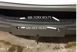
6. PLACE THE BULL BAR IN PLACE USING THE SUPPLIED FASTENERS (ITEM #8,9&10). THE BOLT AND WASHER WILL BE PLACED ON THE OUTSIDE WHILE THE FLANGE NUT WILL FASTEN FROM THE INSIDE. ONCE ALL THE FASTENERS ARE IN PLACE POSISTION THE BULL BAR AND TIGHTEN THE FASTENERS DOWN TO 25 FT LBS.
