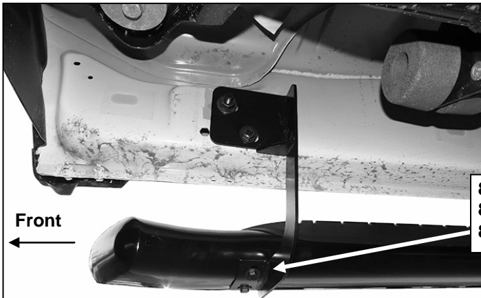
(Fig 15) Passenger/right front Bracket installed
