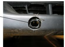
4. INSTALL THE BRACKET (ITEM #2) THROUGH THE BOTTOM HOLES USING THE TWO 7/16"-14 X 3-1/4" HEX SCREWS (ITEM #7), 7/16"-14 SERRATED FLANGE NUTS (ITEM #12) AND THE 3/4" X 2-7/16" SPACERS (ITEM #5). SNUG UP BOLTS TO HOLD THE MOUNTING BRACKET IN POSITION.
