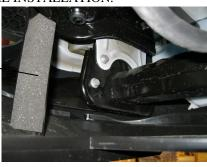
2. LOCATE THE TWO HOLES IN THE LOWER CROSS BRACE AS SHOWN IN *fig. 3.* FROM THE BACKSIDE, USING THE CENTER OF THE CROSSBRACE HOLES AS A GUIDE, DRILL A 1/4" DIAMETER HOLE THROUGH THE PLASTIC BUMPER COVER. (BUMPER COVER REMOVED FOR CLARIFICATION).
