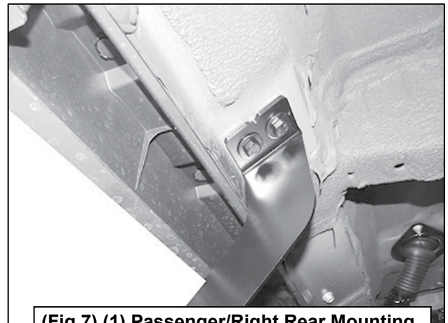
(Fig 7) (1) Passenger/Right Rear Mounting Bracket attached to the 3rd location
