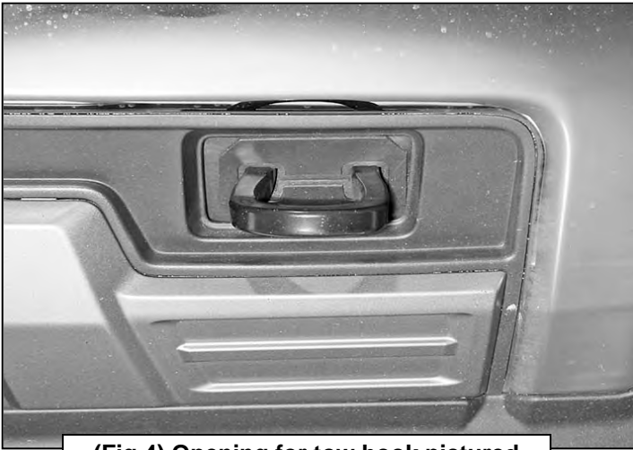
(Fig 4) Opening for tow hook pictured
