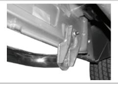
On the driver-side front location remove the factory tape covering the mounting slots in the rocker panel.
