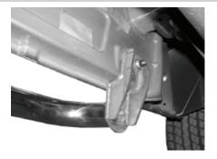
With both the front and rear brackets attached to the rocker panel, remove the front passenger-side factory body bolt. Select the passenger-side front support bracket. Insert the factory body bolt through the support bracket and up into its original position.
