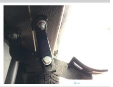
Insert the M10 bolt plate into the access hole in the rocker panel.
