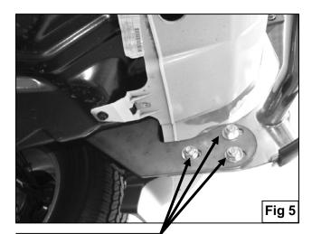
12-1.75mm x 30mm Hex Bolts 12mm Lock Washers 12mm Hex Nuts 12mm Flat Washers
