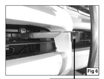
10mm x 25mm Hex Head Bolt 10mm Lock Washer 10mm Hex Nut 10mm Flat Washer
