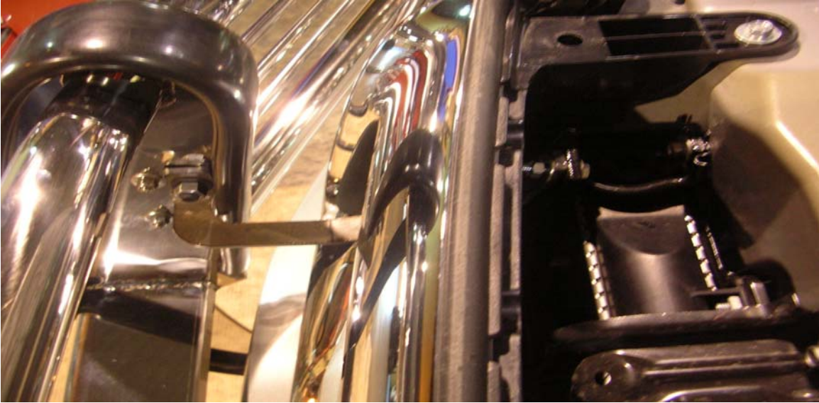
Diagram number 4. Brace bracket installed through grill opening
