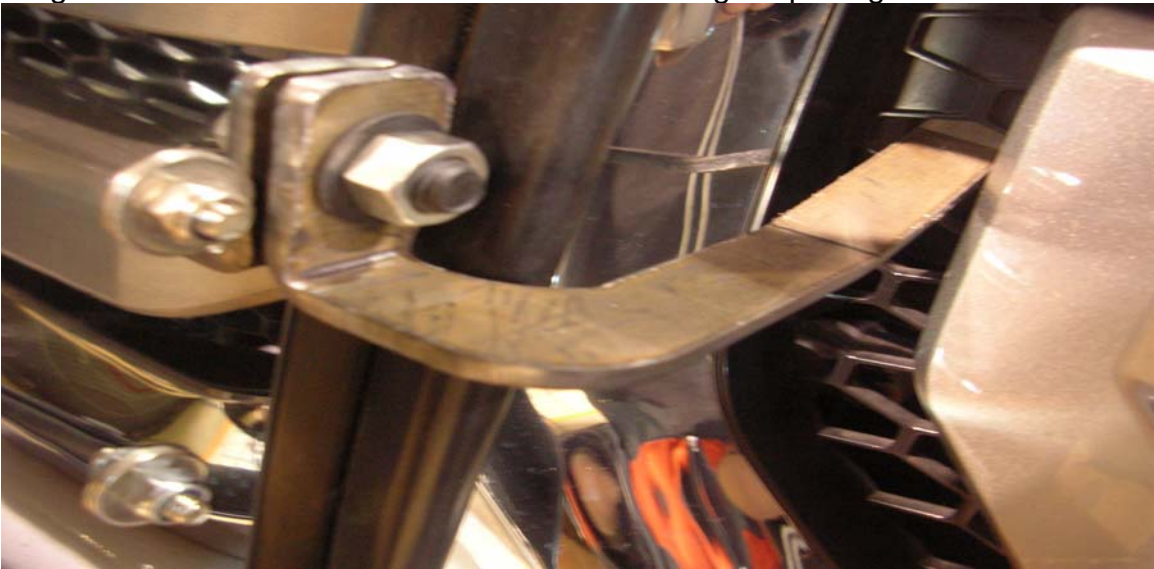
Diagram number 4. Brace bracket installed through grill opening
