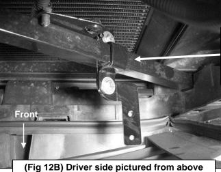
Bolt the Top Inner Bracket to the Backing Plate with:
