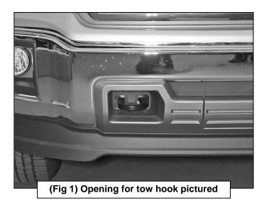
Remove the bolts securing the driver side of the bumper to the bumper bracket. Use a large screwdriver or pry bar to move the mounting tab up enough to get the long bolt through the tow hook out of the end of the frame
