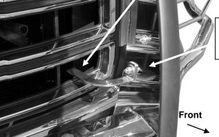
(Fig 17) Driver side outer Top Bracket pictured
