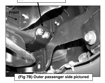
12mm Bolt Plate 12mm Flat Washer 12mm Lock Washer 12mm Hex Nut
