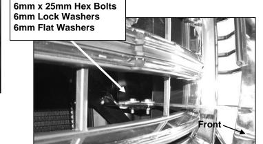
(Fig 16) Driver side Top Bracket
