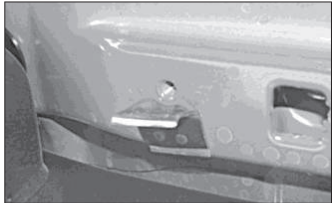
(Fig 2) 8mm threaded hole in floor frame channel (passenger side-front pictured for example)
