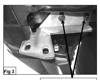
Replace factory bolts with the included: 12-1.25 x 35mm Hex Bolts 12mm Lock Washers 12mm Flat Washers
