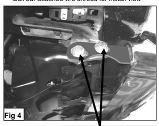
12-1.75mm x 35mm Hex Bolts 12mm Lock Washers 12mm Hex Nuts 12mm Flat Washers
