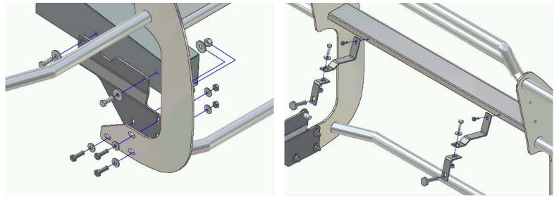
Figure 1.2 – Passenger-Side Mount Bracket
