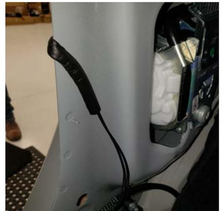
Once the harness and sensor are routed to the desired locations, wipe the sensor and door with the provided alcohol wipe. Place the 3/4" x 1" double-sided tape on the sensor and attach the sensor to the vehicle underneath the door latch. Remove the adhesive back on the foam wire cover and route where desired.
