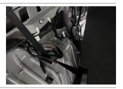
Once the trim panels are removed, take the second section of wiring harness and route it through the driver door sill into the back seat. Route the passenger side of the harness under the carpet below the front of the rear seats.
