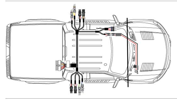
Lift the carpet near the back of the front seat and locate and remove the vent plug. Route the driver-side actuator (red/black) and LED light (brown/tan) wires through the floor and outside of the vehicle. Reinstall the vent plug.
