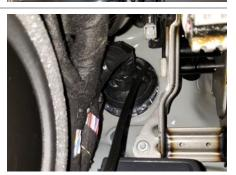
On the driver side of the vehicle remove the door seal, door sill trim panel, the dashboard A pillar trim panel and the kick panel.
