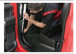
Once the trim panels are removed, take the second section of wiring harness and route it under the carpet, through the vehicle, from the passenger-side rear to the desired location.
