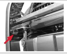
Once the grille guard is aligned, tighten all hardware.
