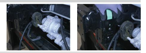
Set the winch support bracket in place making sure the wiring harness is routed below the bracket as shown.
