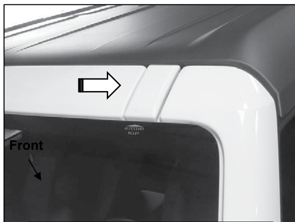
(Fig 1) Remove cover and inner clip
