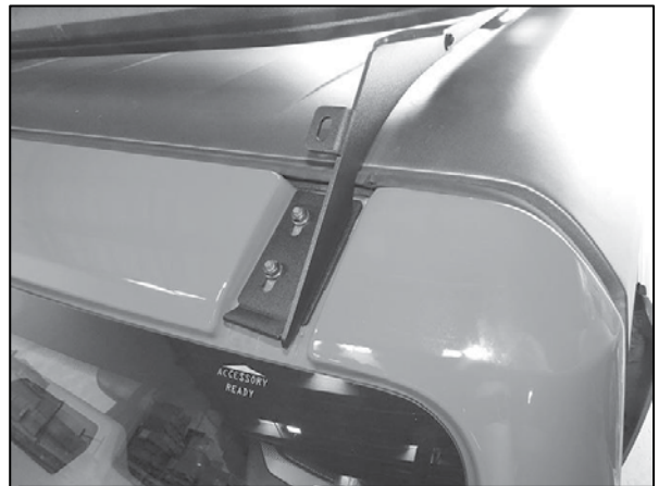
(Fig 21) Attach front mounts to threaded studs and Spacers above front windshield
