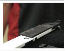
Using the 25mm wide foam tape, apply to the vehicle along the edge of the vehicle back to the rear door.
