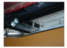
Attach the running board to the brackets using six M8 bolts, lock washers, flat washers and nuts.
