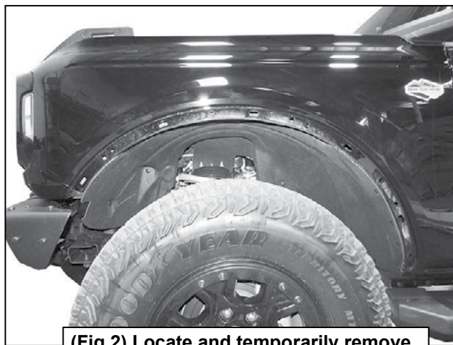
(Fig 2) Locate and temporarily remove the hardware attaching the fender liner to the edge of the wheel well
