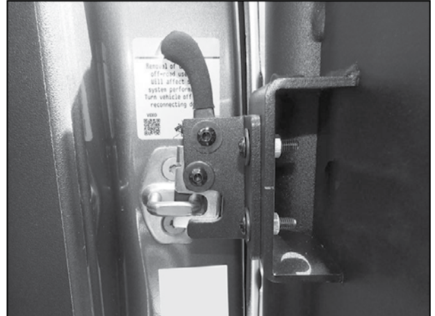
(Fig 16) Adjust Door and Latch assembly for proper operation before fully tightening hardware. Make sure door latch fully closes against striker
